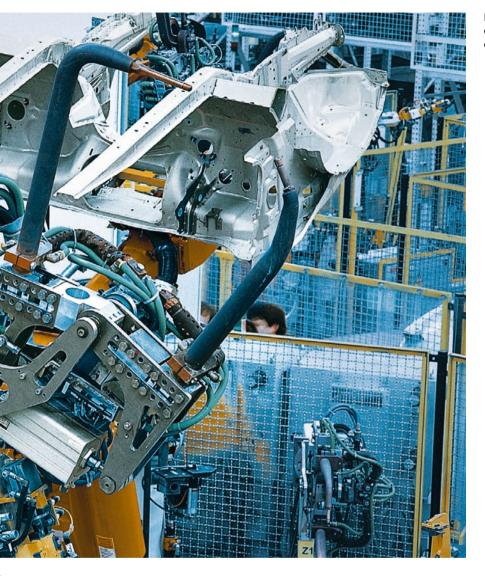
Free choice: servo-pneumatically or servo-electrically driven welding guns.
