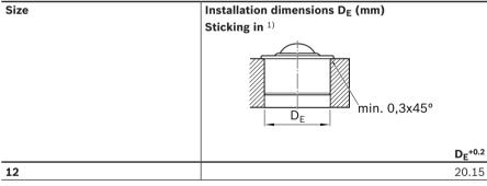
1) For small gap dimensions in metal, we recommend single-component acrylate adhesive. Two-component acrylate adhesives are also possible. The technical data sheets of the manufacturer must be observed.
