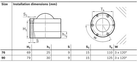
Ball Transfer Unit with solid steel housing R0533 ..., with polymer wiper seal
