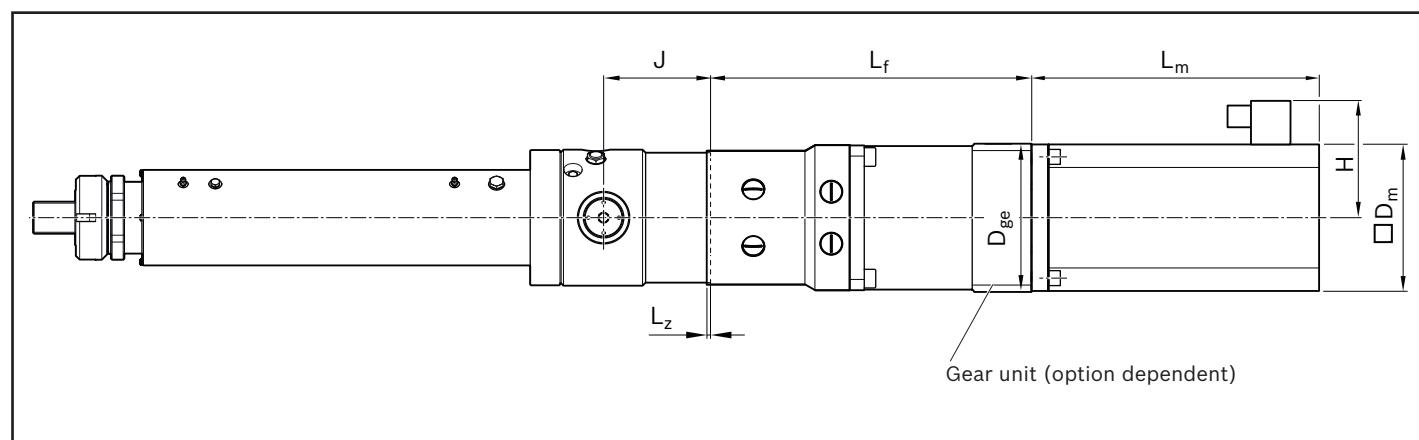
**Note:** The drawing for motor attachment flange and coupling is schematic. Detailed contours can be found in the CAD model.
