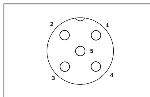
Connection diagram for force measuring bolt
