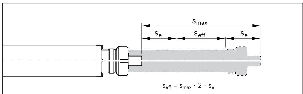
For structural design reasons the overall length of the cylinder is greater than the maximum travel ( $s_{max}$ ), as it includes the length of components such as the screw drive nut or the bearings, in addition to the travel.
