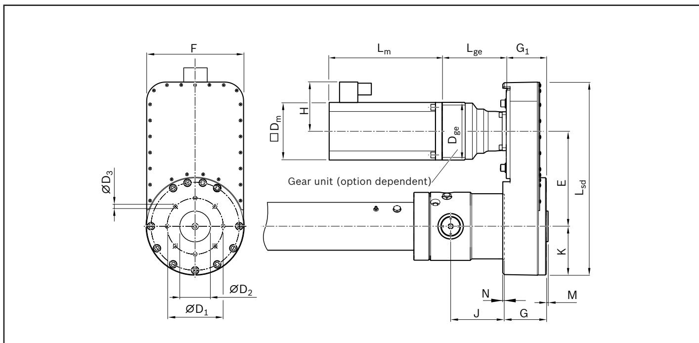
**Note:** The drawing for motor attachment with timing belt side drive is schematic. Detailed contours can be found in the CAD model.
