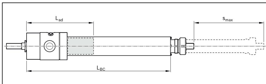
The cylinder can be adapted to the available installation space by mounting the motor as an extension to the axis (mount and coupling) or parallel to the axis (timing belt side drive). The type of motor attachment chosen also has an effect on the technical performance data and the selectable mounting methods.
