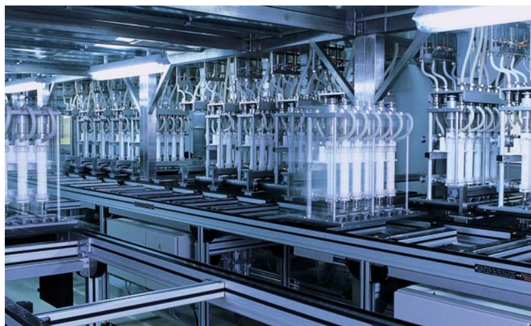
Efficient production of dialysis filters driven by Rexroth TSplus precision assembly conveyor system.
