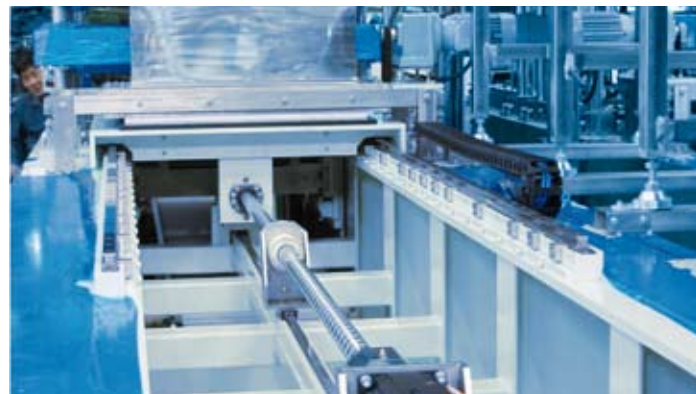
Filling system feed unit for soup powder, double ball rail system on both sides for precise and highly dynamic operation of the unit, powered by a centrally positioned precision ball screw drive
