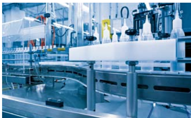
The hygienic VarioFlow stainless steel system transports empty shampoo bottles flexibly and securely to the filling and sealing station
