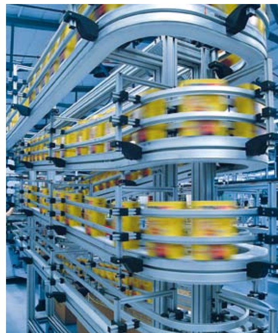
Transport and storage in a single system. With controlled speeds, the VarioFlow system adjusts to the production variations of the machines.
